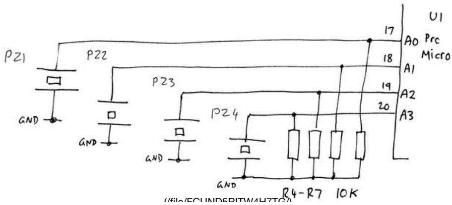
Each pad is connected directly to one of the Arduino's analog inputs (A0-A3), with a 10K resistor connected to ground as shown. You'll need a connector of some sort to allow the pads to be unplugged while assembling the rest of the board.
