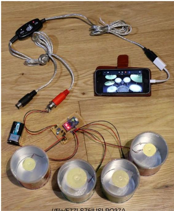
With a bit of luck, you can plug it straight in to a MIDI drum synth and start playing. The four pads transmit kick drum, snare, closed hi-hat and open hi-hat note values according to the General MIDI specification (see "General MIDI Level 1 Percussion Key Map" at <https://www.midi.org/specifications/item/gm-level-1-sound-set> ).
