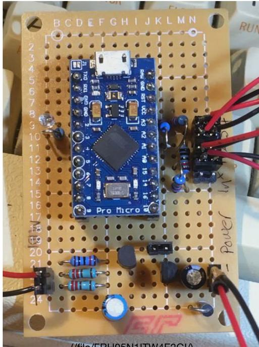
The circuit is simple enough to put together on a breadboard, but I've made a soldered version for robustness. The complete schematic is attached as file *midi-trigger.pdf*, but you may find it easier to construct in individual stages, as shown in the following three steps.
