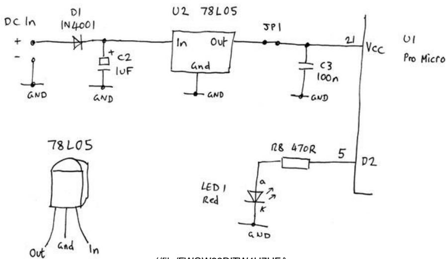
You can power the Arduino over its USB connection, plugging it in to a computer or a power bank. For maximum portability, though, I added a simple voltage regulator to run it from a 9V (PP3) battery. Current drain is about 50mA, so if you're going to use it a lot a rechargeable PP3 is a good idea. I included a removable jumper (JP1) so the regulator circuit can be disconnected when the Arduino is being powered from USB during programming.
